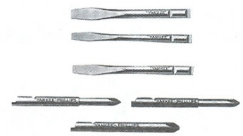
Figure 10-21. The spiral-ratchet screwdriver can be fitted with different types and sizes of bits.
