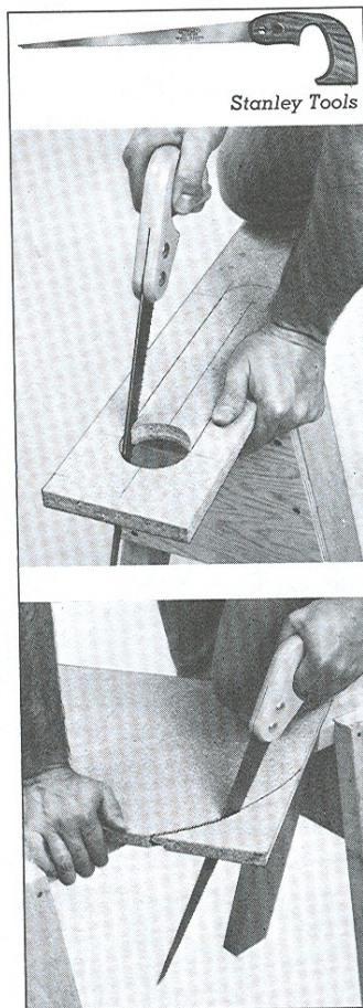
Figure 11-5. A compass saw is used to make curved cuts.
