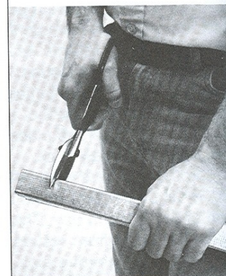
Figure 11-20. Tin snips are used to cut metal framing members.
