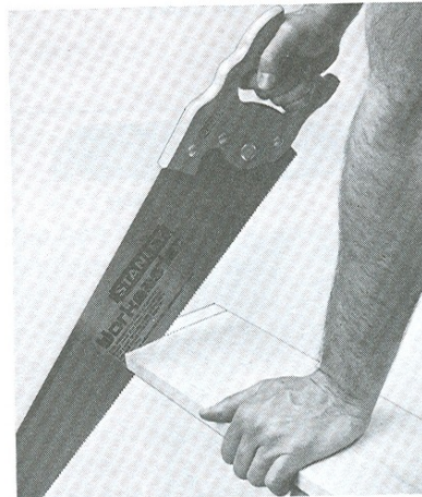
Figure 11-13. Move non-sawing hand a safe distance away from blade after making beginning saw kerf.
