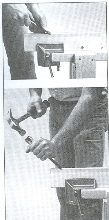
Figure 11-16. When using a wood chisel, keep free hand out of the way of the chisel, and cut away from body.
